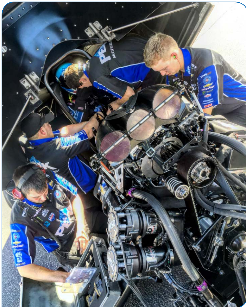
The blower on John Force's record-setting NHRA Funny Car is powered by a synchronous belt drive that helps the 8,000-horsepower dragster exceed 300 miles-per-hour in less than 4 seconds.
